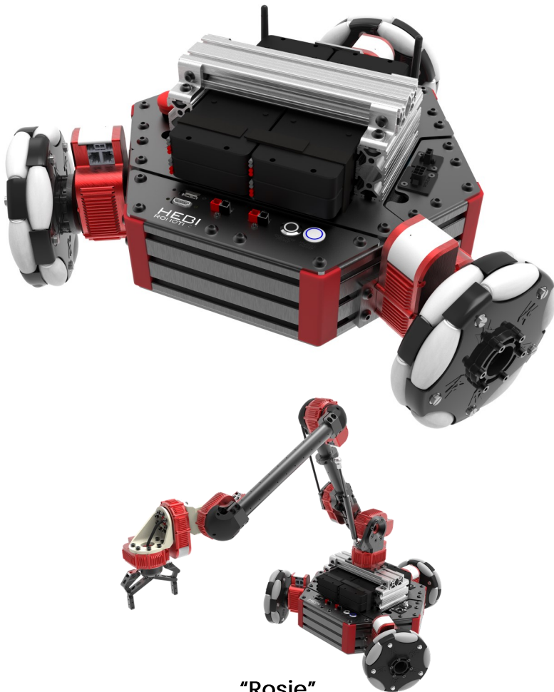
"Rosie" Omni-Directional Mobile Base w/ 6-DoF Arm and Gripper
