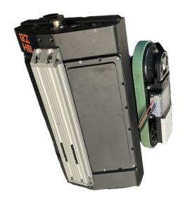
The chassis and actuators on Mack have been tested and operated in shallow water, allowing the robot to be used in pipes and reservoirs without requiring them to be fully drained.
