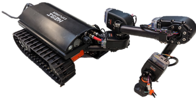
Integrated with 4-DoF Arm and UT Thickness Probe
