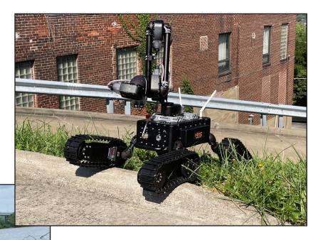
It was initially developed in response to a customer's need for a lightweight and extensible platform to inspect difficult terrains, including landslides. Since then it has evolved into multi-purpose platform capable of performing inspection and maintenance tasks in the most difficult environments and confined spaces.
