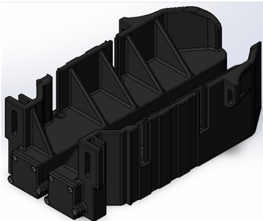
Figure 2. Isometric view of magnetic attachment assemblies in Maggie Robot.
