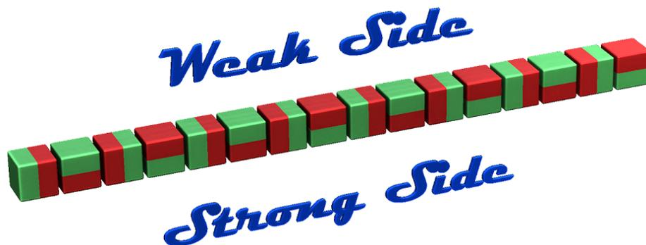
Figure 1. Illustration of magnets arranged in a Linear Halbach Array.
