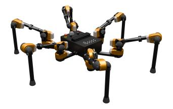
The T-Series Actuator® is designed to function as a full-featured robotic component as opposed to a simple servo motor. The output rotates continuously, requires no calibration or homing on boot-up, and contains a thru-bore for easy daisy-chaining and wiring. This enables these actuators to be used in everything from wheeled robots to multi-degree of freedom collaborative robotic arms.
