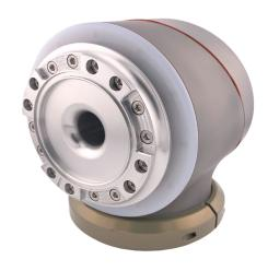
The H-Series Actuator is a full-featured robotic component as opposed to a simple servo motor. The output rotates continuously, requires no calibration or homing on boot-up, and contains a thru-bore for easy daisy-chaining of wiring. This enables the actuators to be used in everything from wheeled robots to collaborative robotic arms.
