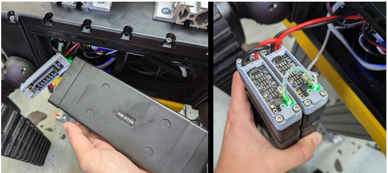
4. Install the batteries back into the cavity with the covers.
