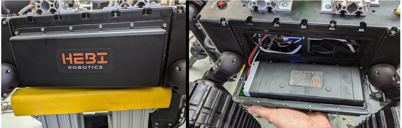
2. Remove the side cover and carefully take the batteries down from the side cavity in the chassis.
