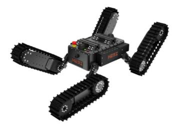
The R-Series Actuator is a full-featured robotic component as opposed to a simple servo motor. The output rotates continuously, requires no calibration or homing on boot-up, and contains a thru-bore for easy daisy-chaining of wiring. This enables the actuators to be used in everything from wheeled robots to collaborative robotic arms.
