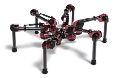
The X-Series module is designed to function as a full-featured robotic component as opposed to a simple servo motor. The output rotates continuously, requires no calibration or homing on boot-up, and contains a thru-bore for easy daisy-chaining and wiring. This enables these modules to be used in everything from wheeled robots to multi degree of freedom collaborative robotic arms.
